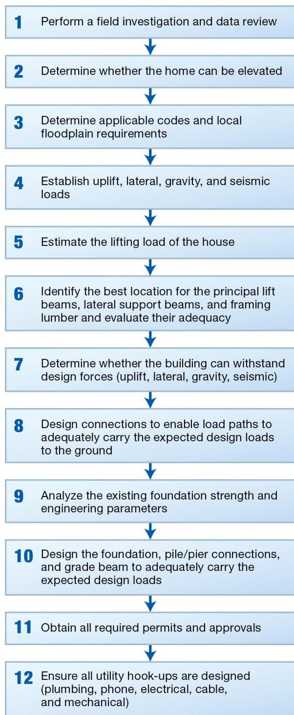
Figure 9: 12-step design process for elevating homes.
