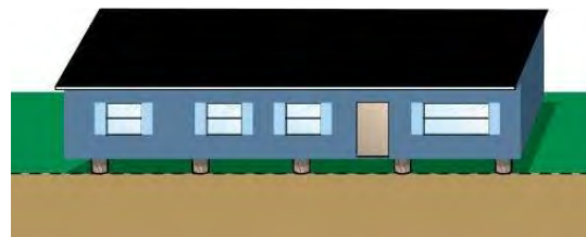
Piers and posts
